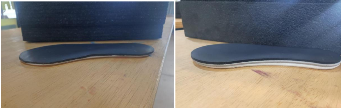
Figure 6: Coated Insoles: (a) Insole coated with a single layer of PORON® 4701-40, and (b) Insole coated with two layers: EVA and PORON® 4701-40. Source: Developed by the authors.
