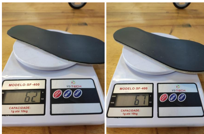
Figure 7: Insole weighing: (a) weight of the single-layer insole, and (b) weight of the double-layer insole. Source: Developed by the authors.
