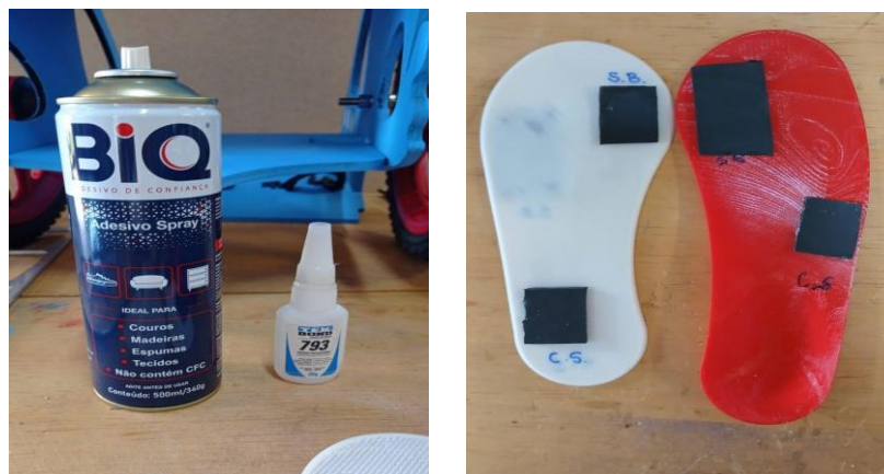
Figure 5: Adhesion test: (a) Tested adhesive glues, and (b) Insoles with the test performed. Source: Developed by the authors.
