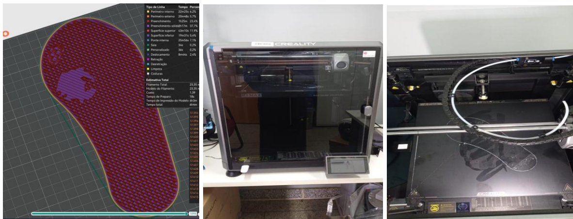
Figure 3: (a) Insole slicing in the OrcaSlicer software. (b) Creality K1 MAX printer, and (c) Insole printing in progress. Source: Developed by the authors.
