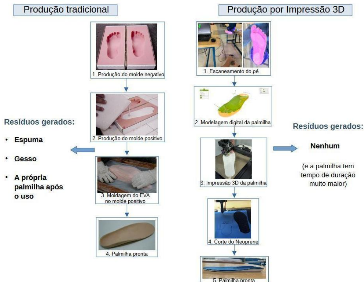
Figure 8: Flowchart of traditional production and rapid prototyping printing. Source: Ribeiro et al. , 2024
