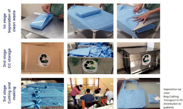
Figure 4: SMS upcycling process captured in operating rooms. Source: Authors (2022).
