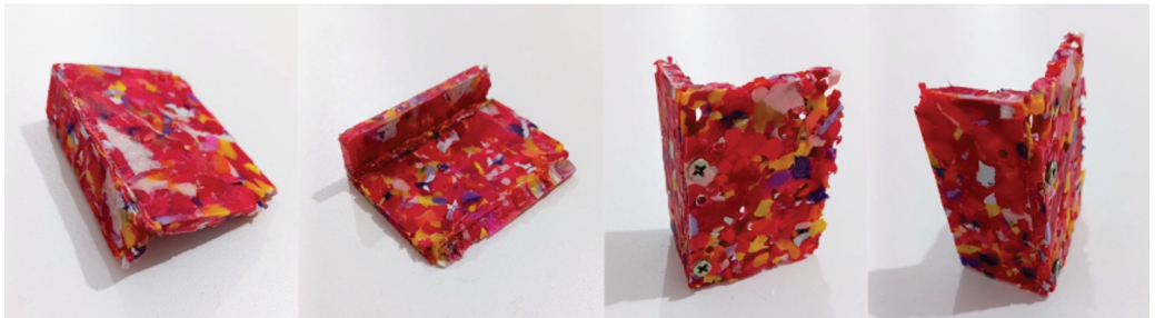
Figure 10 – Welding and screwing tests.
