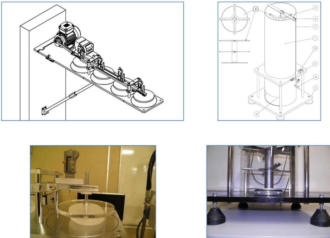
**Figure 2.** Schematic drawing and manufactured equipment details of fatigue (left) and impact (right) equipment developed and patented by the LEBm/HU-UFSC (Source: LEBm/HU-UFSC)
