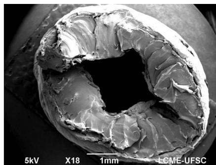
**Figure 7.** Image of the failed surface obtained using MEV of the PLDLA 70/30 interference screw after torsion test (Source: LEBm/HU-UFSC)
