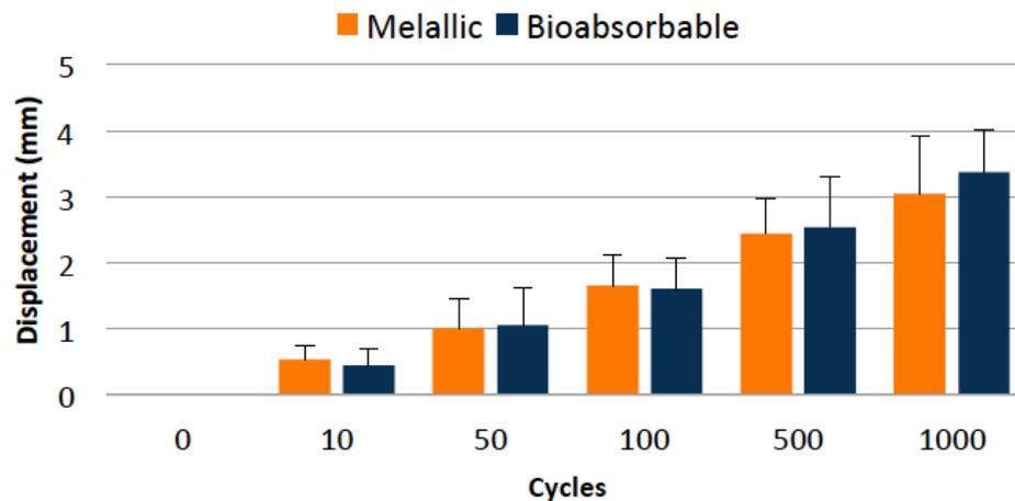
**Figure 4.** Change in length of the graft system/ fixture/tibia after 1000 cycles for two different implants reviews (surgical techniques) (Source: LEBm/HU-UFSC)
