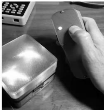
Figure 2. Lighting box to synchronize the transition between asanas among deaf students.
