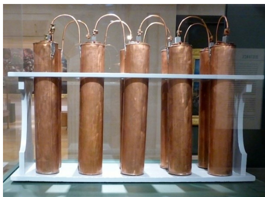
Image 7 – Association of Daniell cells for telegraph networks. Source: < http://www.victorianweb.org/painting/reviews/decoded1.jpg >. Accessed on June 1st, 2021.
