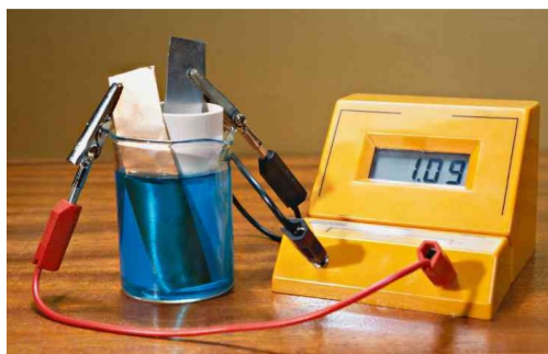
Fig. 3 – Photograph of the assembly of a Daniell Cell. Source: F2, p. 217.
