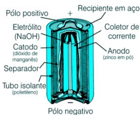
Fig. 9 – Schematic drawing of a MnO_2/Zn alkaline battery. Source: Bocchi et al. (2000, p. 6).
