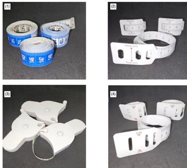
Figure 1. Examples of measuring tapes used to analyze their accuracy and measure the head circumference (HC). Note. Tape 1 (Flexible measuring tapes), 2 (Brazilian HC measuring tape), 3 (telescopic body measuring tape), and 4 (European HC measuring tape).
